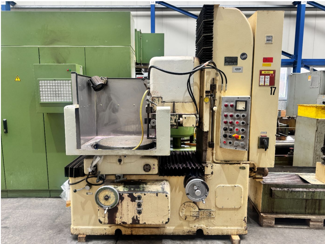
Fig. 1 · Kehren & Co Rotary table surface grinding machine
