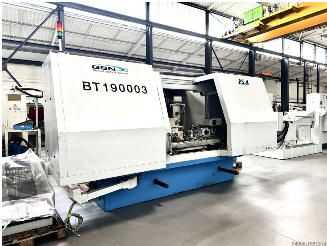
Fig. 1 · Schaudt PS 4 CNC Cylindrical Grinding Machine (Retrofit 2020)
