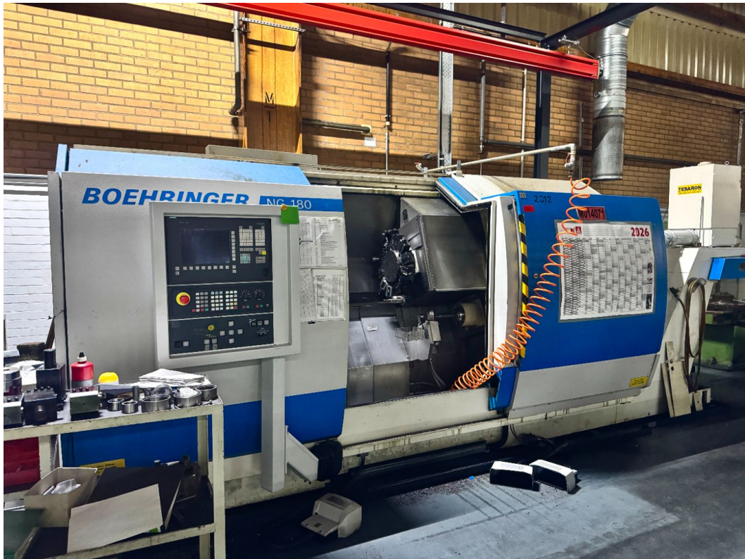
Fig. 1 · VDF Boehringer NG 180 -2 Turning Machine
